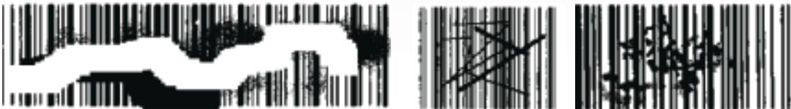
These bar codes were successfully read by the barcode module and could not be read with a hand scanner.
